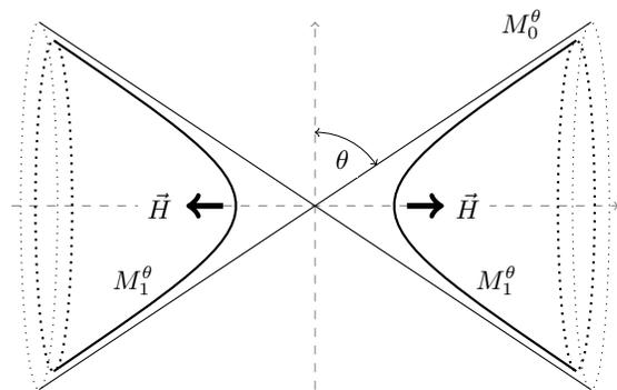
a. The two-sheeted evolution of  $M_0^\theta$  exists for any angle  $\theta$ . It is the unique evolution of  $M_0^\theta$  for  $\theta > \theta_C^*$  and corresponds to the droplets bouncing off each other.
