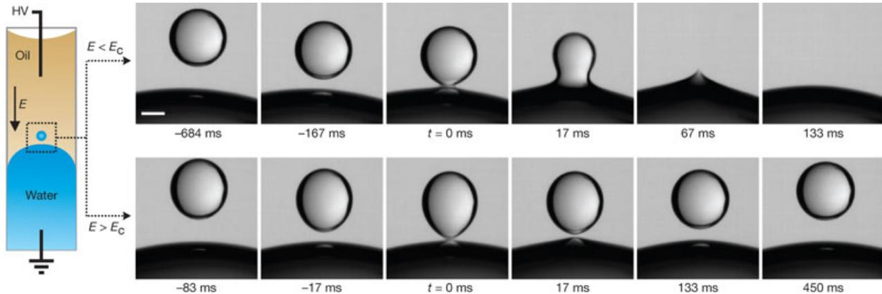
A high-voltage (HV) provides the electric field of strength  $E$ . The top row of images shows coalescence ( $E < E_C$ ) whereas the bottom row shows bouncing ( $E > E_C$ ) of the water droplet. Reprinted by permission from Macmillan Publishers Ltd: Nature, WD Ristenpart et al. **461**, 377-380, ©2009, doi:10.1038/nature08294.
