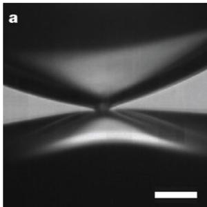
As the droplets touch, they are locally conical, and form a thin connecting bridge. Reprinted by permission from Macmillan Publishers Ltd: Nature, WD Ristenpart et al. **461**, 377-380, ©2009, doi:10.1038/nature08294.
