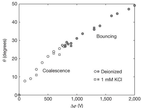
The contact angle  $\theta$  of the double cone for water droplets in air with applied potential  $\Delta\varphi$ . Open symbols denote coalescence, filled symbols denote bouncing. Reprinted by permission from Macmillan Publishers Ltd: Nature, WD Ristenpart et al. **461**, 377-380, ©2009, doi:10.1038/nature08294.
