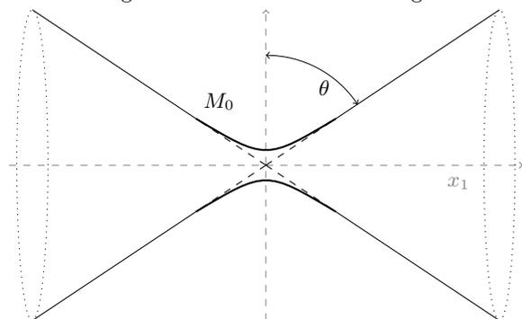
We smooth out the double cone  $M_0^\theta$  in order to obtain a rotationally symmetric surface  $M_0$ , locally modeling the touching fluid droplets.
