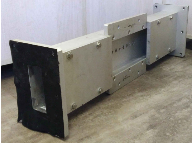
Fig. 2 Photographs of the experimental setup. Top: The impedance eduction duct set up with the the one-sided liner holder [as per 8]. Left: The one-sided liner holder removed from the duct [as per 8]. Right: The two-sided liner holder for the present study. Note that the liners referred to as installed on the “top” and “bottom” surfaces in the text were in practice installed on the left and right of the duct.
