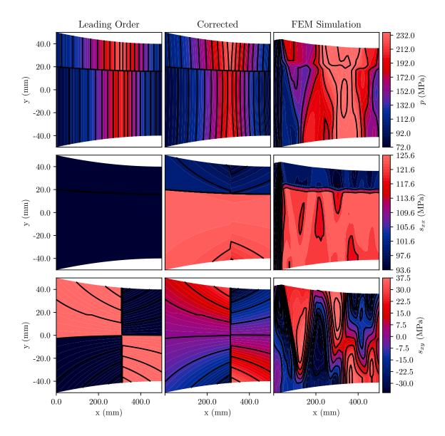
Fig. 3.4 Pressure (top), horizontal deviatoric stress (middle) and shear stress (bottom) fields from the asymptotic model leading order (left) corrected solution (centre) and finite element simulations (right) for  $g_0 = 0.4$  and K = 1.25. The roll set-up is otherwise symmetric with parameters:  $(\hat{h}_0, \delta, r, \mu, \hat{k}) = (0.05, 0.1, 0.20, 0.1, 100 \text{MPa}).$
