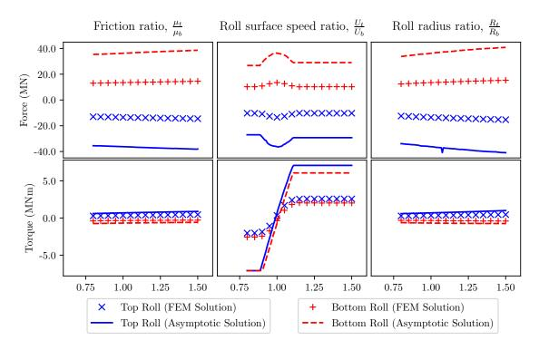
Fig. 5.6 Roll force (top) and torque (bottom) as the top roll is varied to achieve the asymmetric ratio of friction (left), speed (middle) or size (right). The other parameters used are  $(\hat{h}_0, \hat{R}_b, r, \mu, \hat{k}) = (0.01\text{m}, 2.5\text{m}, 0.12, 0.1, 173\text{MPa}).$
