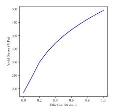
Fig. 2.11 Yield shear stress against effective strain for carbon steel used to compare the present model with ABAQUS simulations. An elastic modulus of 180GPa and Poisson's ratio of 0.27 were also used.
