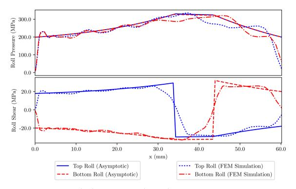
Fig. 2.10 Roll pressure (top) and roll shear (bottom) for the 'Combo 2' parameter set from the corrected asymptotic model and finite element simulations.
