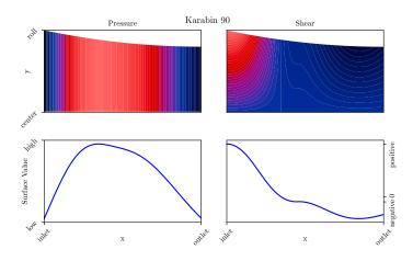
Fig. 1.10 Illustrative example of pressure and shear stress field and respective values on the roll surface for rolling with the Karabin et al. (1990) friction model assuming low friction and a small roll gap aspect ratio.  $\Delta_v = 0.2U_{\text{roll}}, m = 2, l = 2$  and /mu = 0.3.
