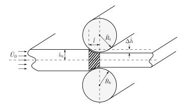
Fig. 1.2 A diagram of rolling illustrating the relevant parameters of two-dimensional geometry. This includes the workpiece half-thickness,  $\hat{h}_0$ ; the roll radii,  $\hat{R}_{t/b}$ , the workpiece inlet velocity,  $\hat{U}_0$ ; the roll gap length,  $\hat{l}$ ; and the gauge,  $\Delta \hat{h}$ .
