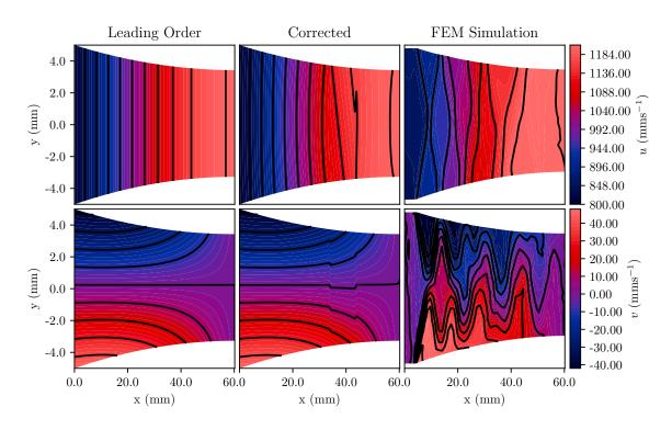
Fig. 2.9 Horizontal (top) and vertical (bottom) velocity fields for the 'Combo 2' parameter set from the asymptotic model; leading order (left) and corrected solution (right).
