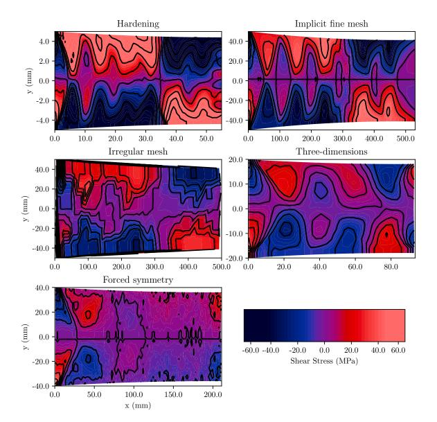
Fig. 5.2 Shear stress fields for a work hardening material, using an implicit finite element solution, using an irregular mesh, for a three-dimensional workpiece, and for the top half of a three-dimensional workpiece with a horizontal plane of symmetry. All cases are symmetric configurations with assorted parameters.
