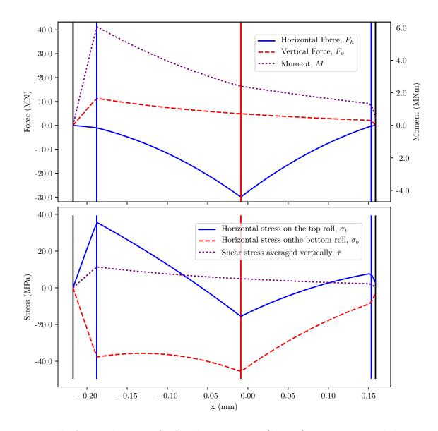
Fig. 6.3 The force and moment (top) and mean stresses (bottom) acting on vertical elements throughout the roll gap. The vertical lines indicate the contact points (black and blue) and neutral points (red). The rolling configuration is defined by  $(\delta, r, k, R_t, R_b, \mu_t, \mu_b, \frac{U_t}{U_b}) = (0.01\text{m}, 0.12, 100\sqrt{3}\text{MPa}, 2.5\text{m}, 2.5\text{m}, 0.1, 0.1, 0.8).$
