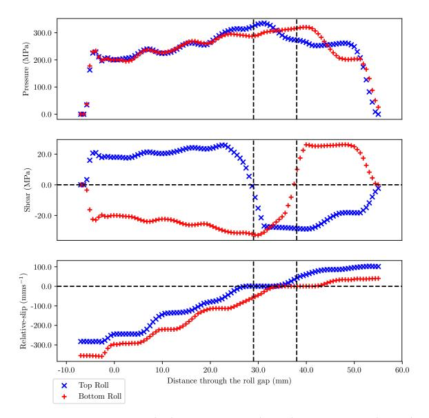
Fig. D.8 Surface normal stress (top), tangential stress (middle) and relative-slip (bottom) throughout the roll gap for an example asymmetric simulation.
