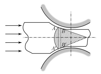
Fig. 1.4 Diagram indicating the approximation of a vertical elemental, A - A' - B' - B, to a compressing wedge solution (shaded) used by Orowan (1943) to close the force balance on each vertical element.
