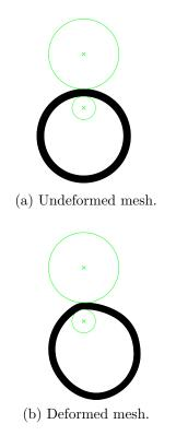
Fig. D.4 Example of the ring rolling mesh used in simulation.
