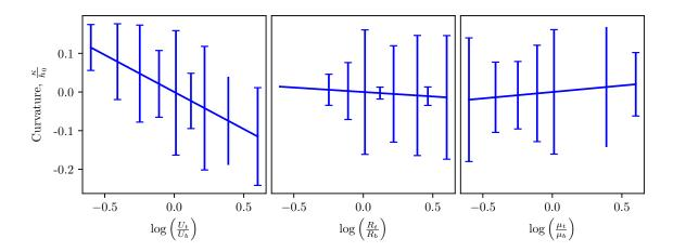
Fig. 4.3 Curvature predictions by the regression model with linear asymmetric terms only. The error bars denote the magnitude of residuals of this model. The rolling set-up is defined by  $(\delta, r, \frac{\sigma_Y}{E}) = (0.3, 0.2, 0.00056)$  and asymmetries in roll surface speed (left), roll size (centre) and friction (right).
