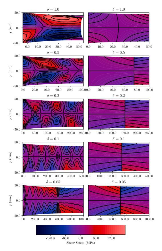
Fig. 5.3 Shear stress fields for varying  $\delta$  from the finite element simulations (left) and the thin-sheet rolling model from Chapter 2(right). The other parameters used are  $(\hat{h}_0, r, \mu, \hat{k}) = (0.05\text{m}, 0.2, 0.1, 173\text{MPa}).$
