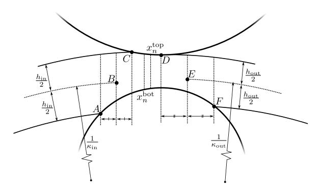
Fig. 6.4 A diagram of the geometry of the roll gap for the ring rolling processes. This illustrates the geometric compatibility of the inner and outer models.
