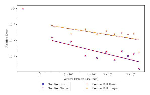
Fig. D.5 Convergence study for the explicit, three-dimensional asymmetric rolling finite element model.
