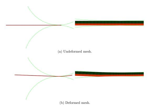
Fig. D.3 Example of clad-sheet rolling mesh used in simulation.
