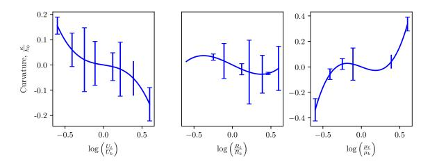
Fig. 4.5 Curvature predictions by the regression model with linear and cubic asymmetric terms multiplied by the material parameter, roll gap aspect ratio and reduction. The error bars denote the magnitude of residuals of this model. The rolling set-up is defined by  $(\delta, r, \frac{\sigma_{\rm Y}}{E}) = (0.3, 0.2, 0.00056)$  and asymmetries in roll surface speed (left), roll size (centre) and friction (right).
