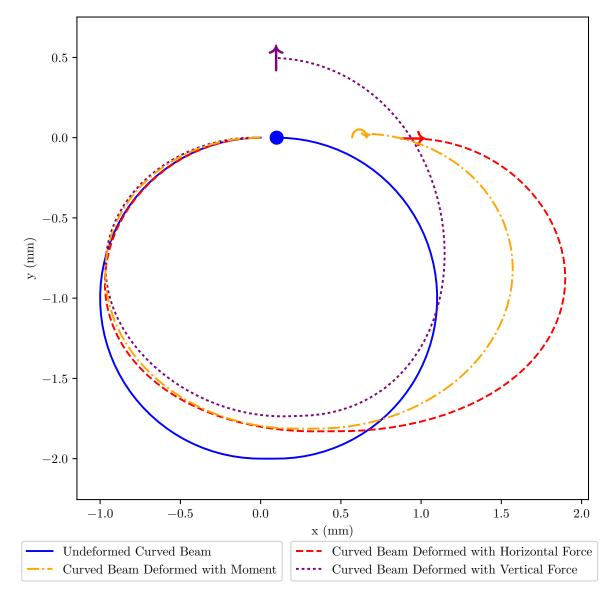
Fig. 6.2 The deflection of an example curved beam under the indicated end forces to illustrate the Timoshenko et al. (1925) curved beam model.
