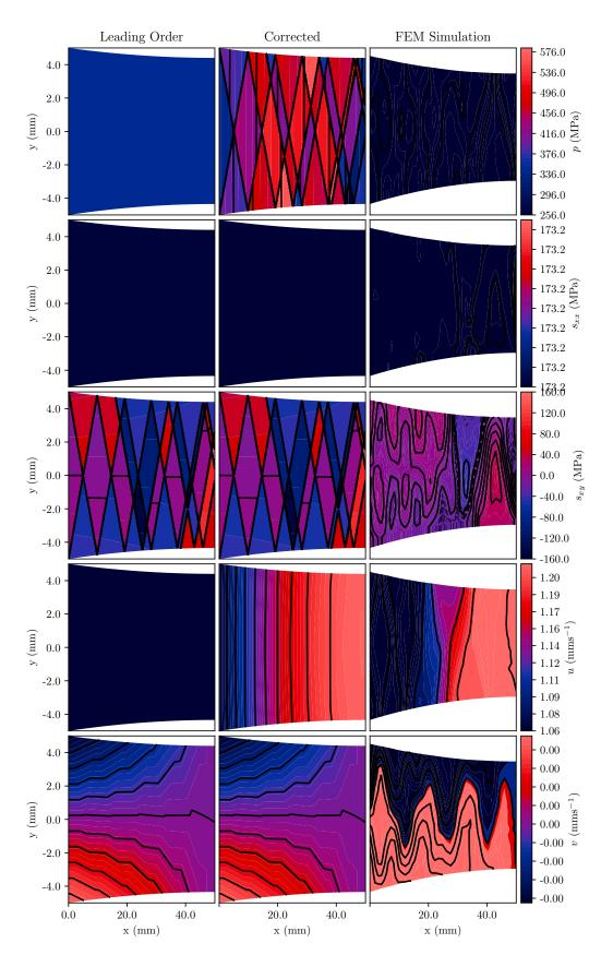
Fig. 5.5 From the top to bottom, pressure, horizontal deviatoric stress, shear stress, horizontal velocity and vertical velocity fields for the for the 'Combo 2' parameter set,  $(\mu_b, \delta, r, \mu_t/\mu_b, \hat{R}_t/\hat{R}_b, \hat{U}_t/\hat{U}_b) = (0.1, 0.1, 0.25, 0.9, 1.1, 0.95)$ , from the leading order asymptotic model (left), corrected asymptotic model (centre) and finite element simulations (right).
