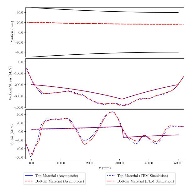
Fig. 3.6 Material interface position (top) and the normal (centre) and tangential (bottom) forces across the material interface for a clad workpiece of  $g_0 = 0.5$  and K = 1.25. The roll set-up is otherwise symmetric with parameters:  $(\hat{h}_0, \delta, r, \mu, \hat{k}) = (0.05, 0.1, 0.20, 0.1, 100 \text{MPa}).$
