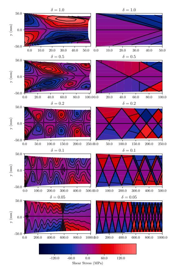
Fig. 5.4 Shear stress fields for varying  $\delta$  from the finite element simulations (left) and the thick-sheet rolling model (right), both exhibiting shear lobes. The other parameters used are  $(\hat{h}_0, r, \mu, \hat{k}) = (0.05\text{m}, 0.2, 0.1, 173\text{MPa}).$
