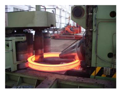
Fig. 1.5 A ring being rolled by a D53K CNC radial axial Ring Rolling Machine. On the left, the ring is pinched between the work roll outside and the mandrell inside. On the right, two horizontal conical rolls prevent vertical growth. Two unpowered guide rolls are also visible on the left, either side of the work roll. As the ring increases in diameter, the left and right sets of rolls are moved apart.
