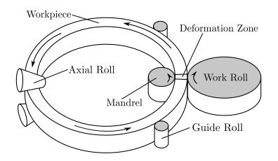
Fig. 6.1 A diagram of the ring rolling process.
