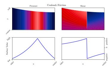
Fig. 1.7 Illustrative example of pressure and shear stress field and respective values on the roll surface for rolling with Coulomb friction assuming low friction and a small roll gap aspect ratio.
