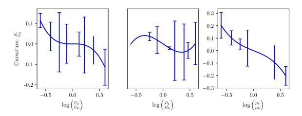
Fig. 4.6 Curvature predictions by the regression model with linear and cubic asymmetric terms multiplied by the material parameter, roll gap aspect ratio and reduction where the probability of the associated coefficient being zero is less than 0.01%. The error bars denote the magnitude of residuals of this model. The rolling set-up is defined by  $(\delta, r, \frac{\sigma_{\rm Y}}{E}) = (0.3, 0.2, 0.00056)$  and asymmetries in roll surface speed (left), roll size (centre) and friction (right).
