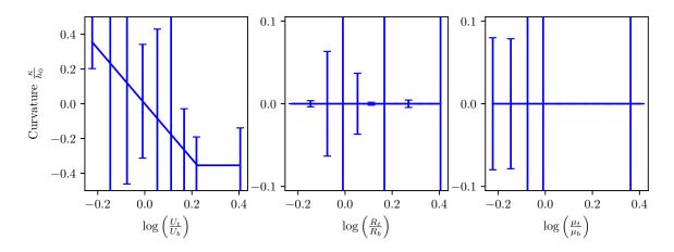
Fig. 4.9 Curvature predictions by the Salimi et al. (2002) model. The error bars denote the magnitude of error between this model and the digitised dataset. The rolling set-up is defined by  $(\delta, r, \frac{\sigma_{\rm Y}}{E}) = (0.3, 0.2, 0.00056)$  and asymmetries in roll surface speed (left), roll size (centre) and friction (right).
