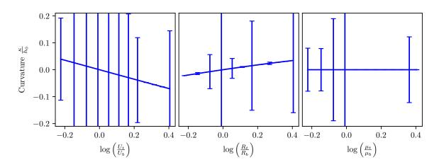
Fig. 4.8 Curvature predictions by the Dewhurst et al. (1974) model. The error bars denote the magnitude of error between this model and the digitised dataset. The rolling set-up is defined by  $(\delta, r, \frac{\sigma_{\rm Y}}{E}) = (0.3, 0.2, 0.00056)$  and asymmetries in roll surface speed (left), roll size (centre) and friction (right).
