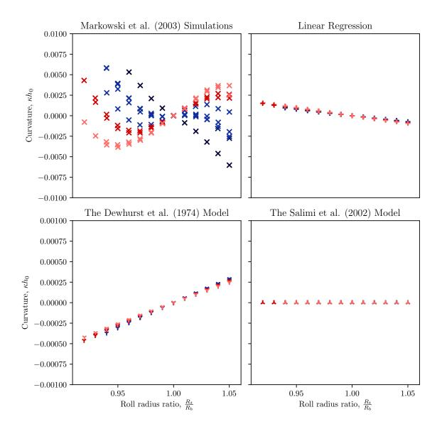
Fig. 4.10 Curvature predictions of the Markowski et al. (2003) simulated results by the reduced cubic linear regression model (top right), the Dewhurst et al. (1974) model (bottom left) and the Salimi et al. (2002) model (bottom right). Colour indicates reduction.
