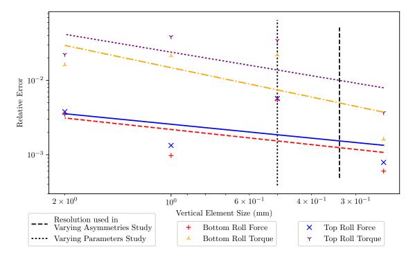
Fig. D.6 Convergence study for the explicit, two-dimensional asymmetric rolling finite element model used in Chapter 2. The discretisation used for the varying asymmetries study and non-dimensional parameters study are marked as vertical long dashed and short dashed lines respectively.
