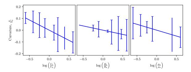
Fig. 4.4 Curvature predictions by the regression model with linear asymmetric terms multiplied by the material parameter, roll gap aspect ratio and reduction. The error bars denote the magnitude of residuals of this model. The rolling set-up is defined by  $(\delta, r, \frac{\sigma_{\rm Y}}{E}) = (0.3, 0.2, 0.00056)$  and asymmetries in roll surface speed (left), roll size (centre) and friction (right).
