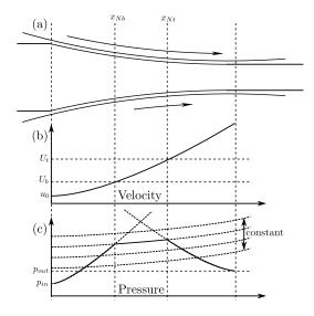
Figure 2: A schematic of the rolling process marking the differences in roll velocity and neutral points (a); a plot of the characteristic surface velocity curve (b); and a plot of the characteristic pressure with alternative, discontinuous, curves as dashed lines (c).
