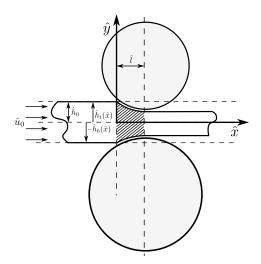
Figure 1: Illustration of the idealised two dimensional rolling model.
