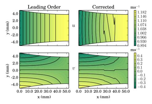
Figure 8: Horizontal (top) and vertical (bottom) velocity fields for the 'Combo 2' parameter set from the asymptotic model; leading order (left) and corrected solution (right).
