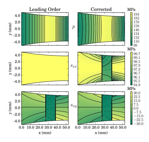
Figure 7: Pressure (top), horizontal deviatoric stress (middle) and shear stress (bottom) fields for the 'Combo 2' parameter set from the asymptotic model; leading order (left) and corrected solution (right). Dashed contours of finer resolution, 0.8MPa, illustrate the behaviour within the cross-shear region.
