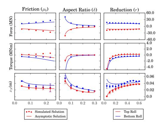
Figure 5: Roll force (top), roll torque (middle) and neutral point (bottom) as the bottom friction magnitude (left), aspect ratio (middle) and reduction (right) were varied for the 'Combo 2' parameter set in Table 1. Error bars indicate the finite length of sticking between the rolls and workpiece.
