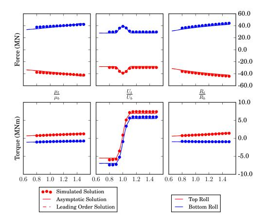
Figure 9: Roll force (top) and torque (bottom) as the top roll is adjusted to vary the ratio of roll characteristics: friction (left), speed (middle) and size (right). The other parameters used are  $(\hat{h}_0, \hat{R}_b, r, \mu, \nu, \hat{E}, \hat{k}) = (0.01\text{m}, 2.5\text{m}, 0.12, 0.1, 180\text{GPa}, 0.27, 186\text{MPa to } 494\text{MPa}).$
