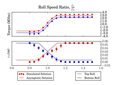
Figure 4: Roll torque (top) and neutral point (bottom) as the top roll speed is varied for the 'perfectly plastic' material. Error bars indicate the finite length of sticking between the rolls and workpiece. The other parameters used are  $(\hat{h}_0, \hat{R}_b, \hat{U}_b, r, \mu, \hat{k}) = (0.01\text{m}, 2.5\text{m}, 1.2\text{ms}^{-1}, 0.12, 0.1, 173\text{MPa})$ . Error bars indicate the finite length of sticking between the rolls and workpiece.
