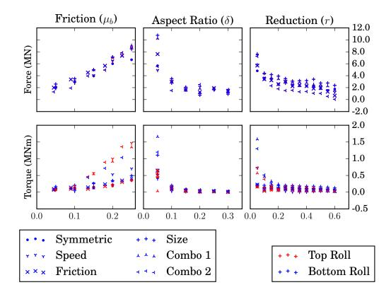
Figure 6: Absolute error in roll force (top) and torque (bottom) between the asymptotic solution and simulation results as the bottom friction magnitude (left), aspect ratio (middle) and reduction (right) were varied for each of the parameter sets in Table 1.
