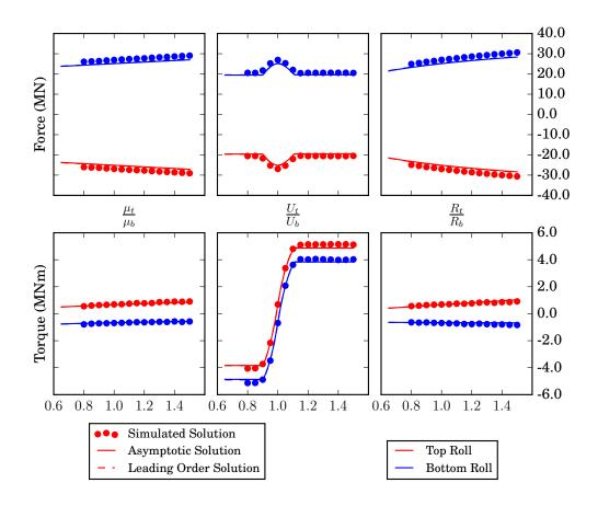
Figure 3: Roll force (top) and torque (bottom) as the top roll is adjusted to vary the ratio of roll characteristics: friction (left), speed (middle) and size (right). The other parameters used are  $(\hat{h}_0, \hat{R}_b, r, \mu, \hat{k}) = (0.01\text{m}, 2.5\text{m}, 0.12, 0.1, 173\text{MPa}).$
