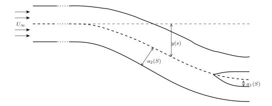
Figure 4.1: Schematic of the duct geometry.
