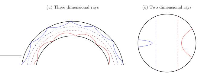
Figure 4.27: Schematic of localized fundamental rays. The dashed lines are where  $\alpha^2 = 0$ . (a) shows the three-dimensional rays, and (b) shows the two-dimensional representation derived in §4.7.1.
