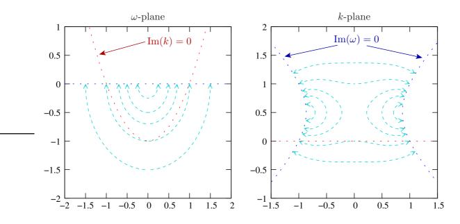
Figure 2.7: Rienstra's (1985) method applied to (2.4) with  $u \equiv 1$ .
