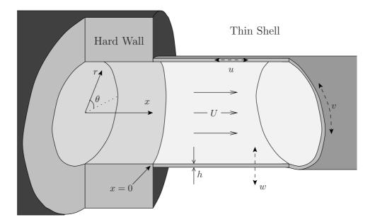
Figure 3.1: Schematic of a cylindrical duct with a sudden change from hard-wall boundary for x < 0 to thin-shell boundary for x > 0. The small unsteady perturbations to the position of the thin shell are given by u, v, and w.
