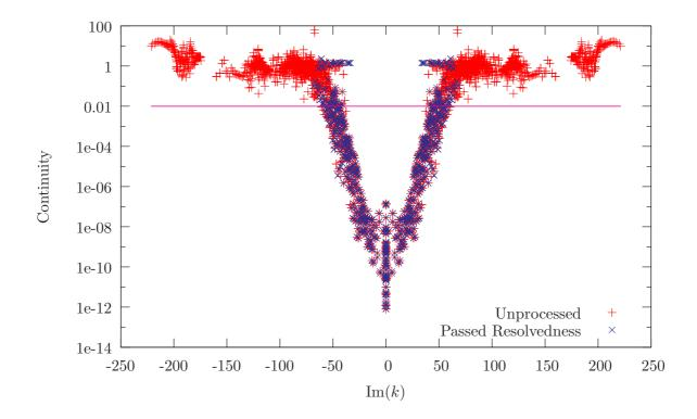
Figure 4.3: Graph showing the continuity of eigenvalues for  $U_{\infty} = 0.5$ ,  $\kappa = 0.1$ ,  $a_1 = 0.4$ ,  $a_2 = 1.0$ ,  $\gamma = 1.4$ ,  $\omega = 10$ ,  $n_r = 21$ ,  $n_{\theta} = 81$ , compared against  $n_r = 25$ ,  $n_{\theta} = 75$  with the same settings.
