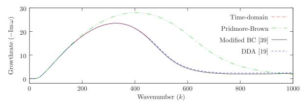
Figure 6: Exponential growth rate as a function of wavenumber for case B, grid 4. The time-domain computational result is obtained from a discrete Fourier transform of the growth between times t = 3.2 and t = 4.5. Also plotted are growth rates given by the discrete dispersion analysis [19], the continuous analytic result using the modified boundary condition [39], and the dispersion analysis from solving the Pridmore-Brown equation resolving the boundary layer.
