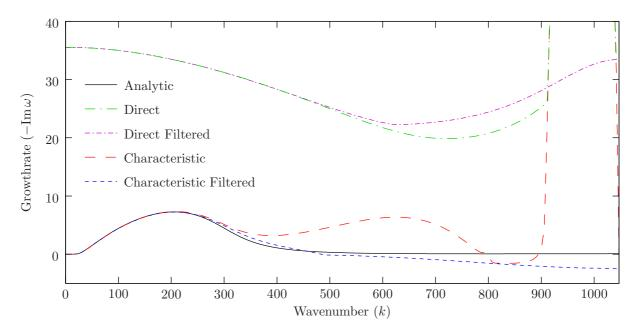
Figure 8: Growth rate against wavenumber for grid 3 of case C for various implementations of the boundary condition. The two curves labelled "direct" apply the boundary condition directly using (12), while the two curves labelled "characteristic" modify the incoming characteristic using (11). In the filtered cases, the n7 filter described in §5 is used.
