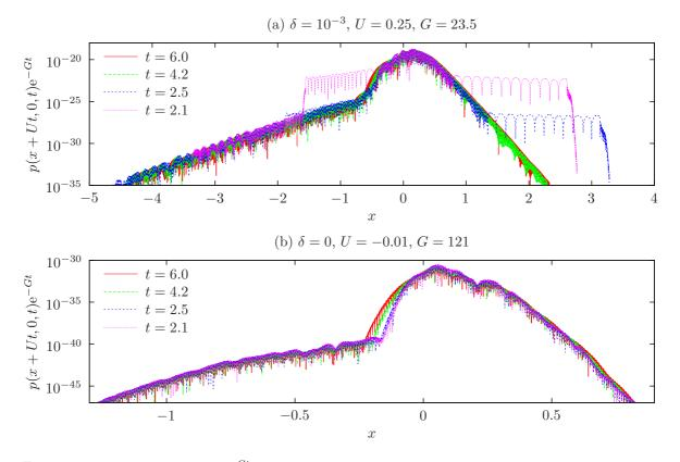
Figure 4: Plots of  $p(x + Ut, 0, t)e^{-Gt}$ , where p(x, 0, t) is the numerically calculated pressure along the lining y = 0 for grid 4 of case B (table 1). (a) includes the boundary layer with incoming characteristic filtered using the n7 filter (section 5). (b) ignores the boundary layer but still filters the incoming characteristic with filter n7. Note that (a) and (b) are plotted using different scales.
