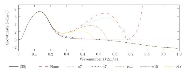
Figure 13: For case C, grid 4, plots of the growth rate  $(-\text{Im }\omega)$  predicted by the DDA [19] against wavenumber k for various filters, together with the analytic solution using the modified boundary condition from Ref. 39.
