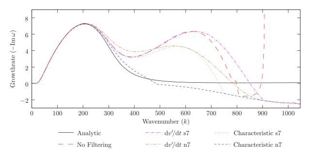
Figure 11: Growth rate against wavenumber for grid 3 of case C, applying the boundary condition using the characteristic method (11), for various different boundary condition filtering schemes. Either the normal velocity derivative dv'/dt or the characteristic amplitude  $\theta$  is filtered using either the mild s7 or strong n7 filters described in §5.
