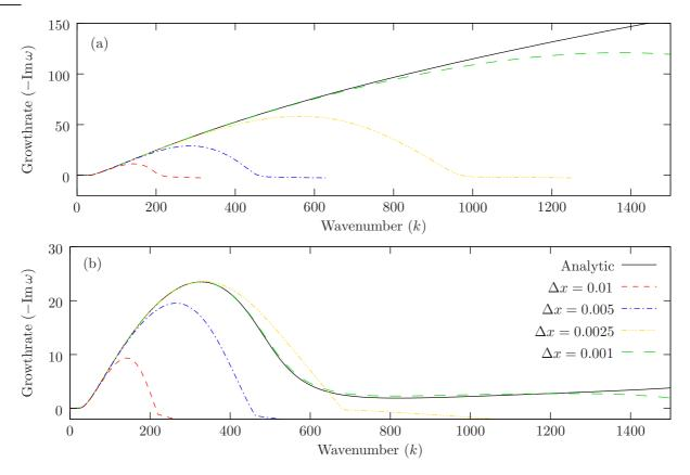
Figure 7: For case B, plots of the growth rate  $(-\text{Im }\omega)$  predicted by Ref. 19 against wavenumber k for various grid resolutions, together with the analytic solution using either the Myers boundary condition [8] or the modified boundary condition from Ref. 39.
