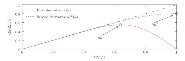
Figure 9: Effective wavenumbers  $\kappa(k)$  and  $\kappa^{(2)}(k)$  for the DRP finite difference derivatives used here. For reference  $\kappa = k$  is also plotted. Circles indicate points where  $d\kappa/dk = 0$  and  $d\kappa^{(2)}/dk = 0$ , given by  $k\Delta x = \alpha_0$  and  $k\Delta x = \alpha_0^{(2)}$  respectively.
