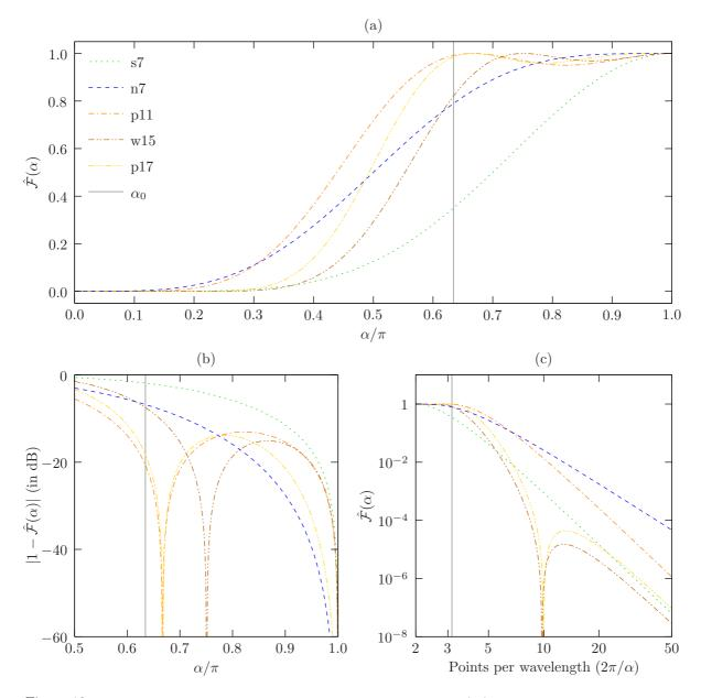
Figure 12: Plots of the response of the filters listed in table 2, defined by (15) with coefficients given in table 3. The vertical line labelled  $\alpha_0$  denotes the position of the zero derivative of the DRP derivative stencil. (a) The overall response of the filter. (b) Overall damping (in dB) at short wavelengths. (c) Effect of damping against number of points per wavelength.
