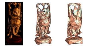
• In order to compute a parameterization (i.e., homeomorphism) between two surfaces of non-zero genus, the first step is generally to cut them open into a disk.
