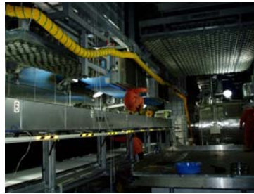
Figure 3. The 10m wind tunnel in the Shinjo Cryospheric Environmental Simulator.
