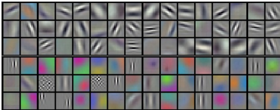
Figure 26.1: Filters for a convolutional layer from an image classification tasks, Krizhevsky et. al.
