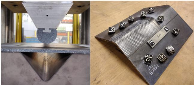
**Fig. 2.** Application of paint patterns for strain analysis. A speckle pattern is applied to the edge and bending punch for DIC analysis, while the circle pattern is applied to the face for CGA analysis.
