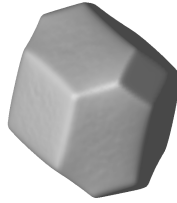
Fig. 13. Building block of the 3D cuboid tiling: A octahedron truncated at the edges in two different portions, revealing 2 small, 4 large square and 8 distorted hexagonal faces.
